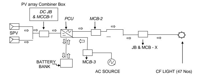
Diagram A: Schematic diagram of the Power Plant
